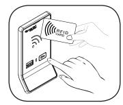
Operate with a User RFID To unlock: Touch I then present an assigned User RFID. To relock: Close the door.
