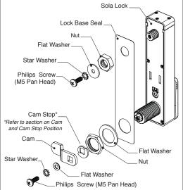
Door thickness: 11-22mm (.433"-.866") Use upper screw hardware
