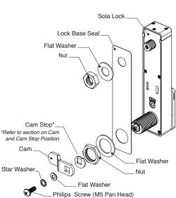
Door thickness: 6-10mm (.236"-.394") Use upper screw hardware
