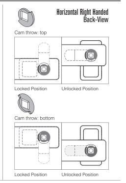
**IMPORTANT:** Do not operate and turn the handle to the unlocked position without first installing the lock or determining whether the lock is for a left or right handed configuration.
